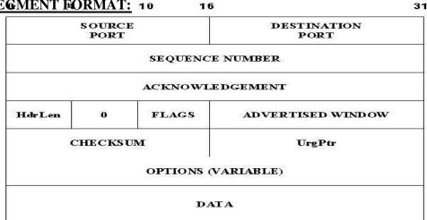
TCP is a byte oriented protocol, which means that the sender writes bytes into a TCP connection and the receiver reads bytes out of the TCP connection. Although "byte stream"
