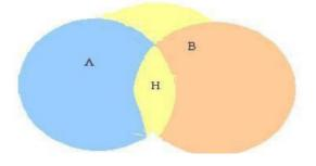
Figure shows that node A and B can each communicate with the H, but are hidden from each other. A situation like this faces two kinds of problems,
