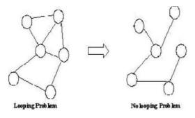
Consider the following extended LAN with many bridges or switch forms loops. If we remove some ports for the bridge or switch from the topology, the extended LAN reduced to a cyclic tree. The main idea of the spanning tree is for the bridge or switch to select the ports over which they will forward frame. The algorithm selects ports as follows.
